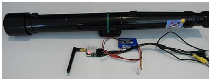
Figure19. Preliminary OptoBotics wireless video systems. Top left photo shows a 2.4 GHz transmitter / Camera driven by a standard 9 V battery viewing a white target screen with rulings. The bottom left photo shows a 5.8 GHz wireless transmitter / receiver with the image (of a flower) taken through the Galileoscope in the top right photo.
